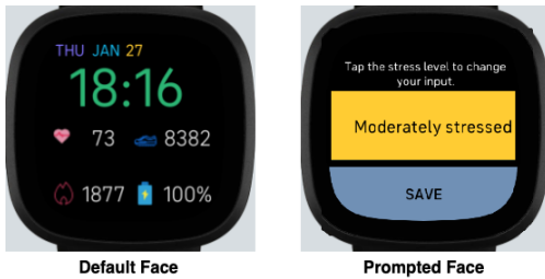
Fig. 2. Custom-built Fitbit clock face built to collect self-reported stress levels from cadets in real-time while also serving general watch functionality with a traditional default face. On prompt, the watch face displays 5 stress levels on a rotating cycle as options for stress reporting from the user.
