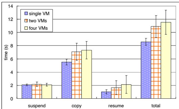
**Figure 8:** The per-VM migration time when different numbers of VMs, each with a 512MB memory, were migrated in sequence. A local disk on the destination host was used to store the migrated VM states.
