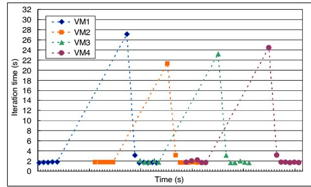
Figure 13: The performance of a memory-intensive benchmark running inside of four VMs that were under migration.
